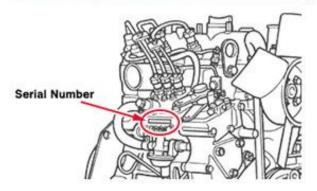
Located on the side of fixing point of injection pump
