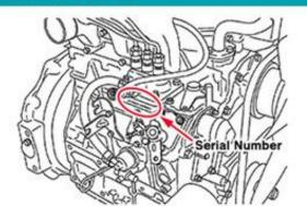
Located on the mounting surface of injection pump
