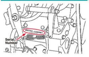
Located on the side of fixing point of injection pump
